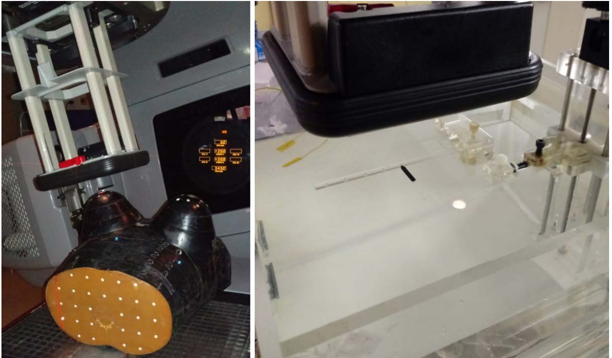
Figure 2 - Experimental setup for the phantom irradiation at left and for TLD calibration curve at right.
